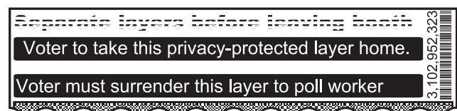
Figure 3. Last inch of the printout after it's separated: (a) the receipt (the layer the voter selects to keep) and (b) the layer that's shredded before the voter leaves the polling place.
