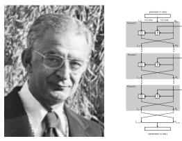
DES Designed at IBM; Horst Feistel supplied key elements of design, such as ladder structure. NSA helped, in return for keeping key size at 56 bits.(?)
