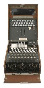
Cryptography performed by (typically, rotor) machines.
