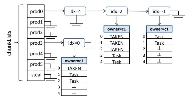
Figure 2: Chunk lists in SALSA single consumer pool implementation. Tasks are kept in chunks, which are organized in perproducer lists; an additional list is reserved for stealing. Each list can be modified by the corresponding producer only. The only process that is allowed to retrieve tasks from a chunk is the owner of that chunk (defined by the ownership flag). A Node's index corresponds to the latest task taken from the chunk or the task that is about to be taken by the current chunk owner.
