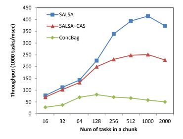
Figure 8: System throughput as a function of the chunk size.
