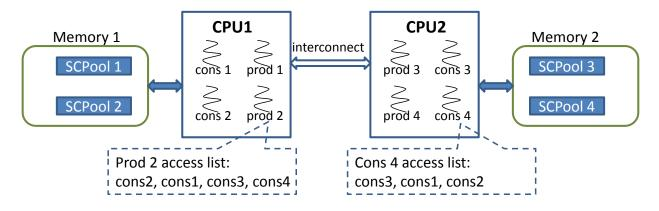
Figure 1: Producer-consumer framework overview. In this example, there are two processors connected to two memory banks (NUMA architecture). Two producers and two consumers running on each processor, and the data of each consumer is allocated at the closest physical memory. A producer (consumer) has a sorted access list of consumers for task insertion (respectively stealing).
