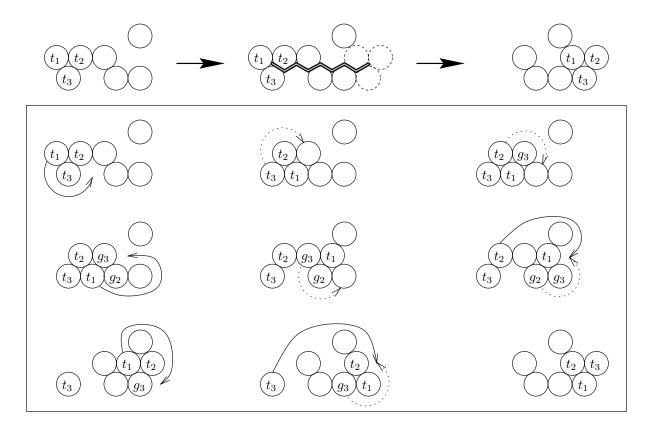
Figure 13: An example of triangle maneuvering. Dotted arrows denote conceptual moves, and solid arrows denote actual moves.
