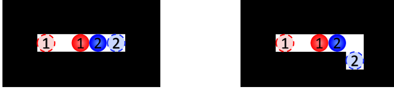
Figure 2: In this image, black cells are fixed, white cells are free, solid discs are individual particles, and goal positions are dashed circles. For the simple instance on the left, it is impossible to maneuver both particles to end at their goals. The instance on the right has a finite solution: \langle r, d, \ell \rangle .
