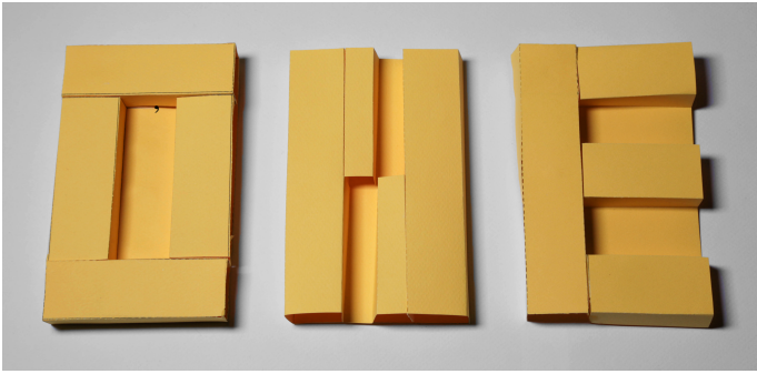
FIGURE 11: REAL-WORLD CONSTRUCTION OF “ONE” USING OUR SINGLE-CUT FONT FROM FIGURE 10. THE MATERIAL IS 98 LB / 160 GSM WATERCOLOR PAPER (SOLD AS MI-TEINTES BY CANSON).
